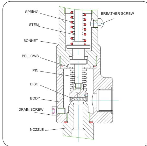
2) A protection bellows protects the spindle, spindle guide and all the safety valve's upper part including the spring from contact with the process fluid, ensuring the integrity of the moving parts and helping to prevent corrosion, abrasion or fluid polymerisation or crystallisation damaging the components located in the upper part of the valve.
